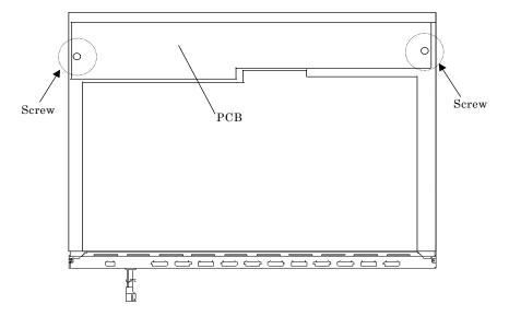
Figure 4-71 Replacing Samsung fluorescent lamp (WXGA) (2)
